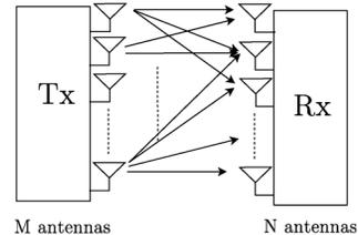
Fig. 1. MIMO: With  $M$  transmitters and  $N$  receivers.
