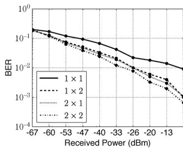
Fig. 3. Measured BER versus SNR for MIMO configurations.
