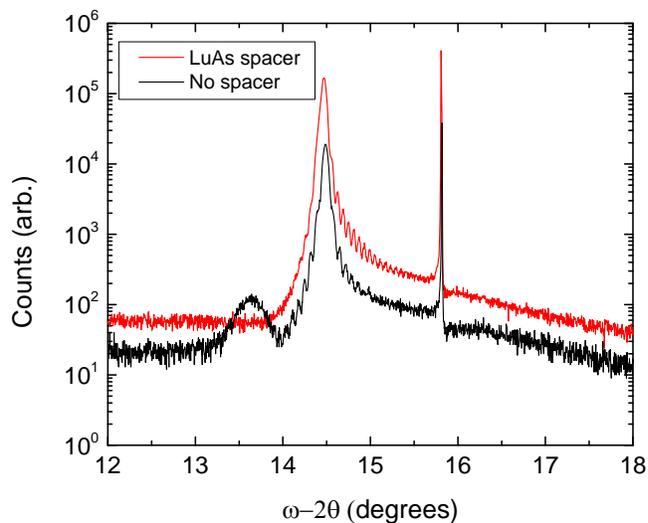
Figure (4): Including a spacer of 10 ML of LuAs separating the LaAs film and the GaAs cap layer removes the side-peak observed in the  $\omega$ - $2\theta$  scan of the samples.
