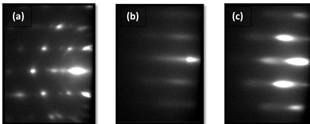
Figure (2): (a) Polycrystalline RHEED pattern during LaAs growth on GaAs (no LuAs seed), (b) 1nm deposition of LaAs on 5 ML LuAs seed, (c) 14 nm deposition of LaAs on 5 ML LuAs seed, spottiness is attributed to roughening of growth surface due to exceeding critical thickness.
