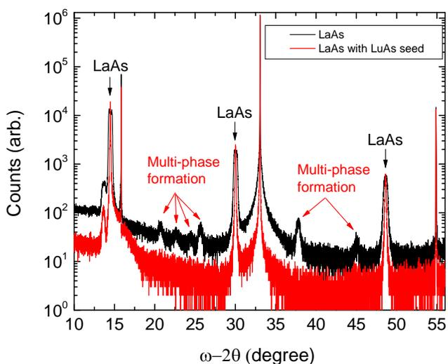
Figure (3):  $\omega$ - $2\theta$  XRD spectra comparing the multi-phase formation occurring in LaAs films grown directly on GaAs substrates versus the LaAs film grown on the 5 ML LuAs seed. Both films were grown at 460°C and 120x arsenic overpressure.
