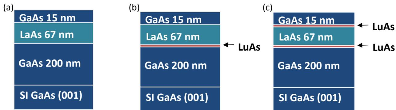
Figure (1): Layer structures: (a) LaAs films on GaAs, (b) LuAs seeded growth 5-10ML of LuAs, and (c) LuAs seeded LaAs film with LuAs diffusion barrier.
