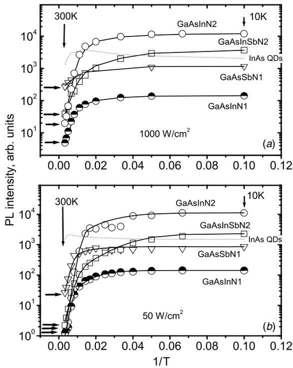
**Figure 4.** The integral intensity of the PL spectra versus temperature (circles, triangles and squares) and an Arrhenius plot fitting (solid curves) for GaAsInN1 (half-filled circles), GaAsSbN1 (inverted triangles), GaAsInSbN2 (squares) and GaAsInN2 (solid circles) QW samples, measured at power density: (a) 1000 W cm<sup>-2</sup> and (b) 50 W cm<sup>-2</sup>. Dashed curves are experimental data for the reference InAs QD sample.
