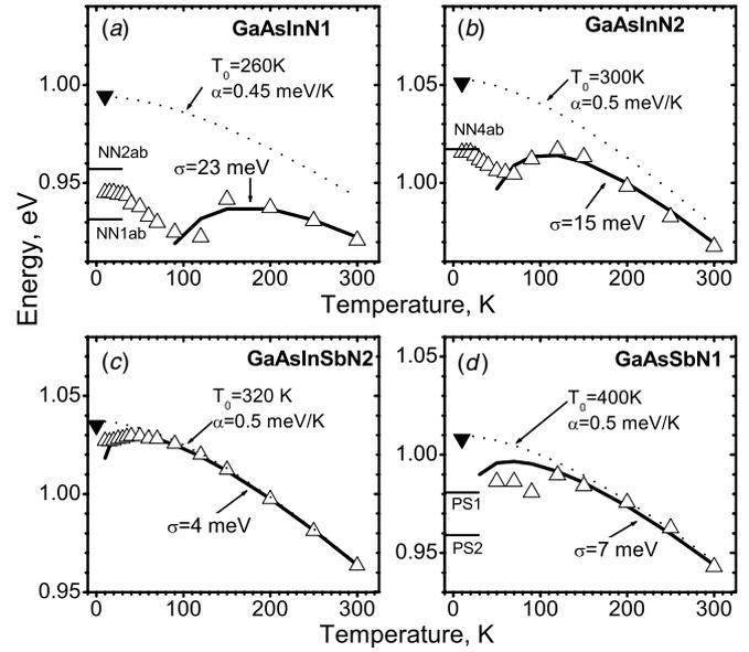
**Figure 3.** Temperature dependence of PL peak position (open triangles), band-tail model [28] (thick solid curves) and the Varshni band-gap model (thin dotted curves) for GaAs(In, Sb)N QWs. The solid inverted triangle at 10 K is the energy  $E_0$  in each case. The horizontal lines are the energies of the fine structure components of the HSR spectra. The power density is  $50 \text{ W cm}^{-2}$ .
