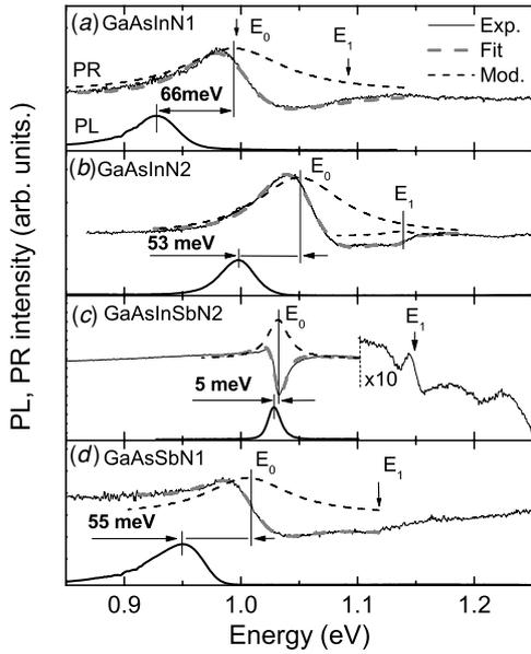
**Figure 2.** Experimental PR and PL spectra (solid curves) of GaAs(In, Sb)N QWs together with PR spectra simulations (thick dashed curves). Thin dashed curves represent the module of the PR resonance transition contribution.
